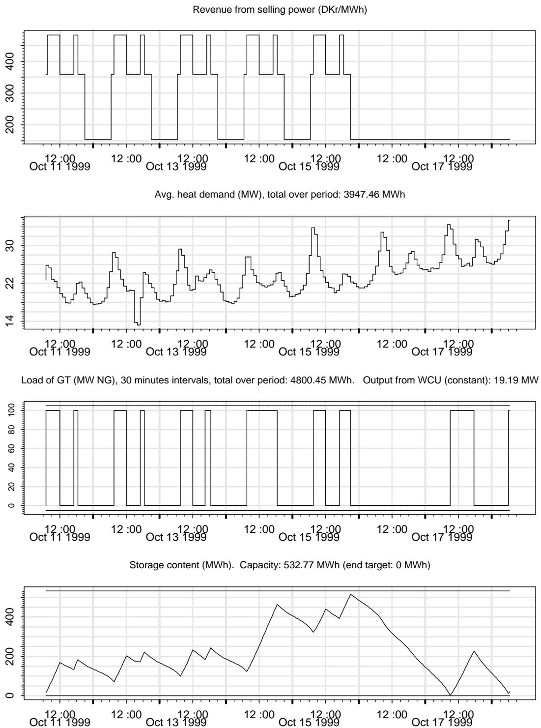
Figure 5.3: Optimal operation of gas turbine for one week starting on 1999.10.11 (criteria function: 631390 DKr).
