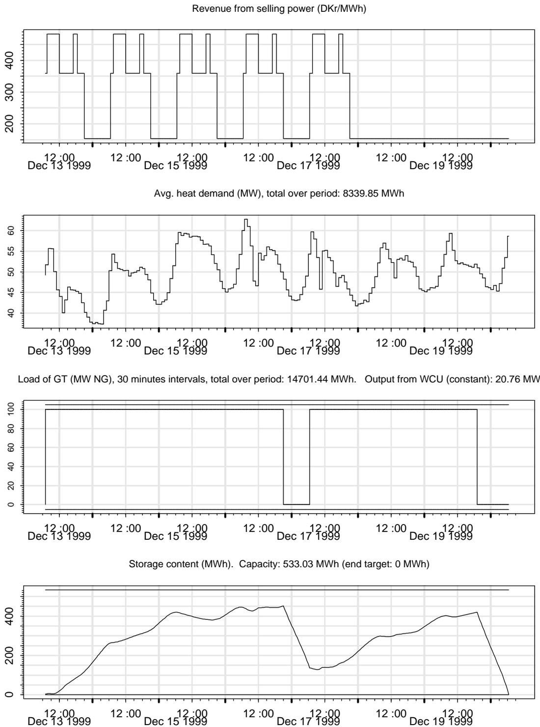
Figure 5.5: Optimal operation of gas turbine for one week starting on 1999.12.13 (criteria function: 940135 DKr).
