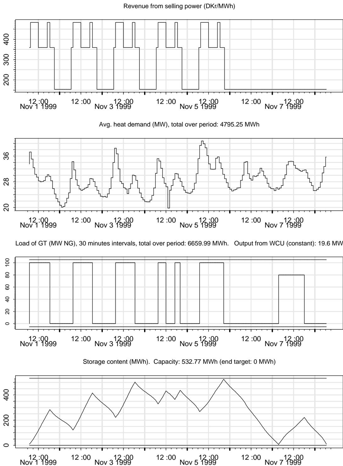
Figure 6.2: Optimal operation of gas turbine for one week starting on 1999.11.01.
