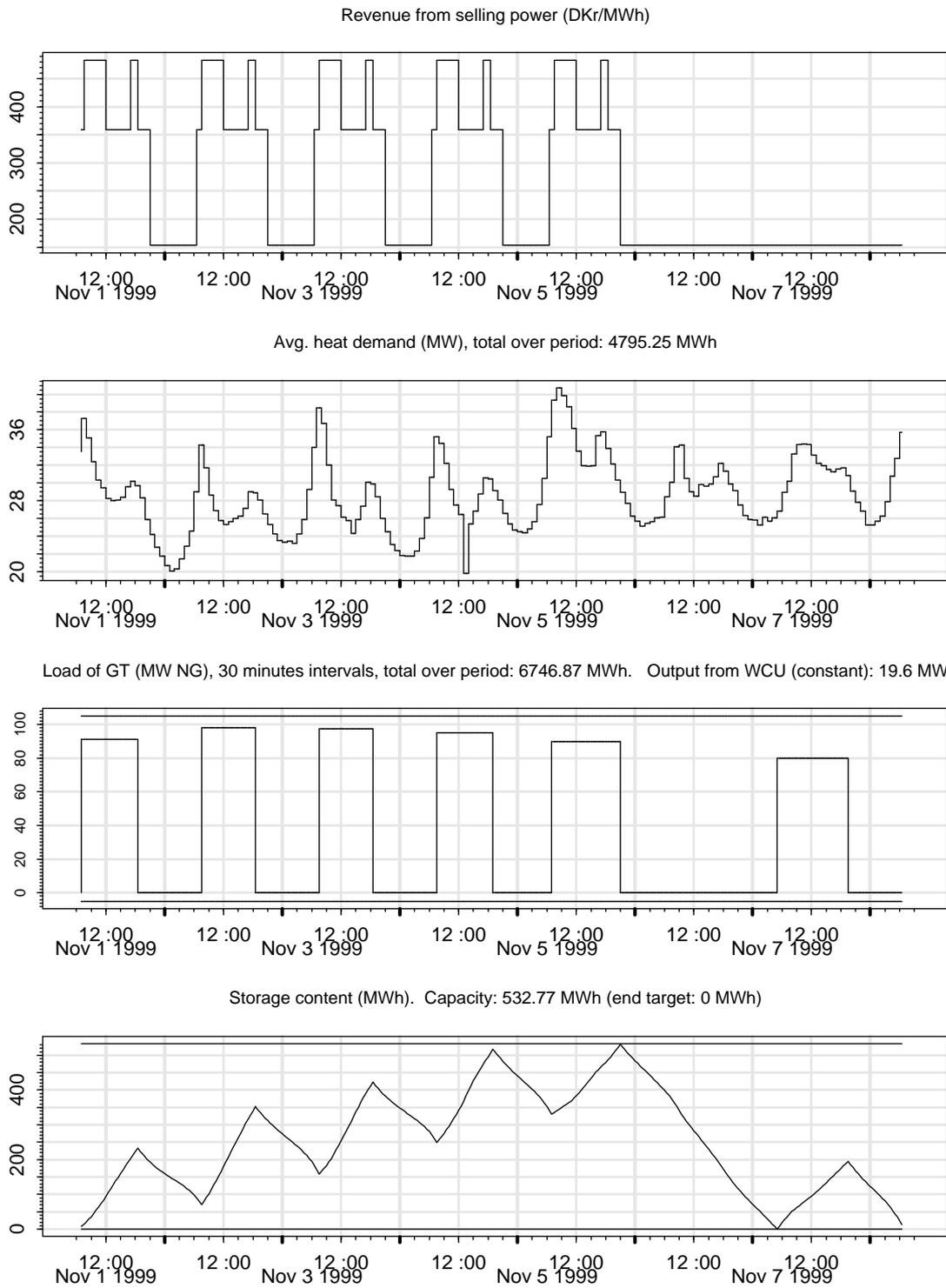
Figure 6.3: Optimal operation of gas turbine for one week starting on 1999.11.01.
