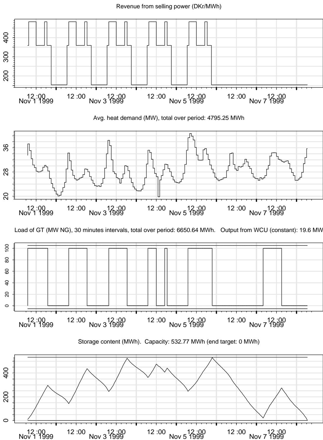
Figure 5.4: Optimal operation of gas turbine for one week starting on 1999.11.01 (criteria function: 793807 DKr).
