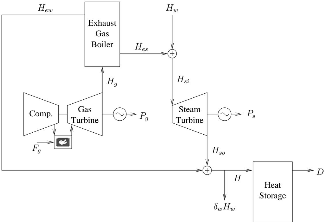
Figure 4.2: Graphical description of the model for Søndersborg CHP plant.
