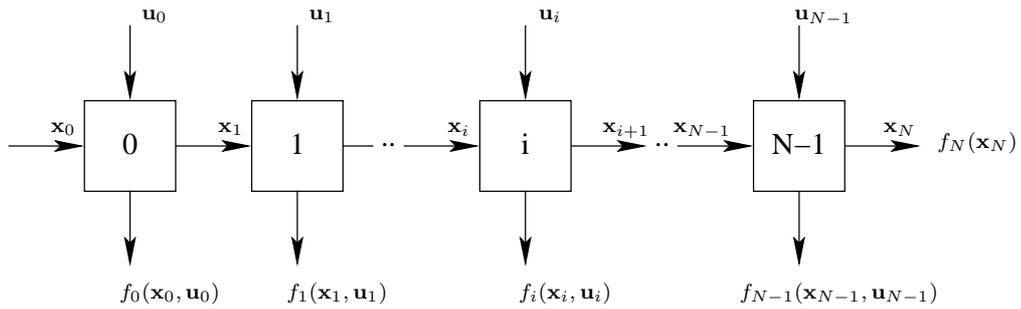
Figure 3.1: Dynamic structure of the optimal control problem.
