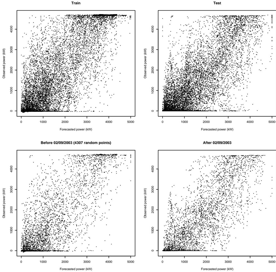
**Figure 4.1:** Observed versus forecasted power (horizons 18-36 hours since 06Z) for the training and test data (top row), and before and after a model change in DMI-HIRLAM which is expected to have large influence on the forecasted 10 m wind (bottom row). Note that the length of the training and test periods are both five months. Also, the two plots in the bottom row contain the same number of points; to achieve this a random subset of the points before the model change is selected.
