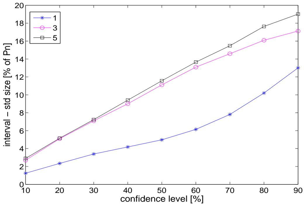
Figure 5.10:  $\sigma$ -diagrams for 24-hour ahead forecasts for evaluating the influence of the power curve mapping on the resulting probabilistic forecasts resolution.
