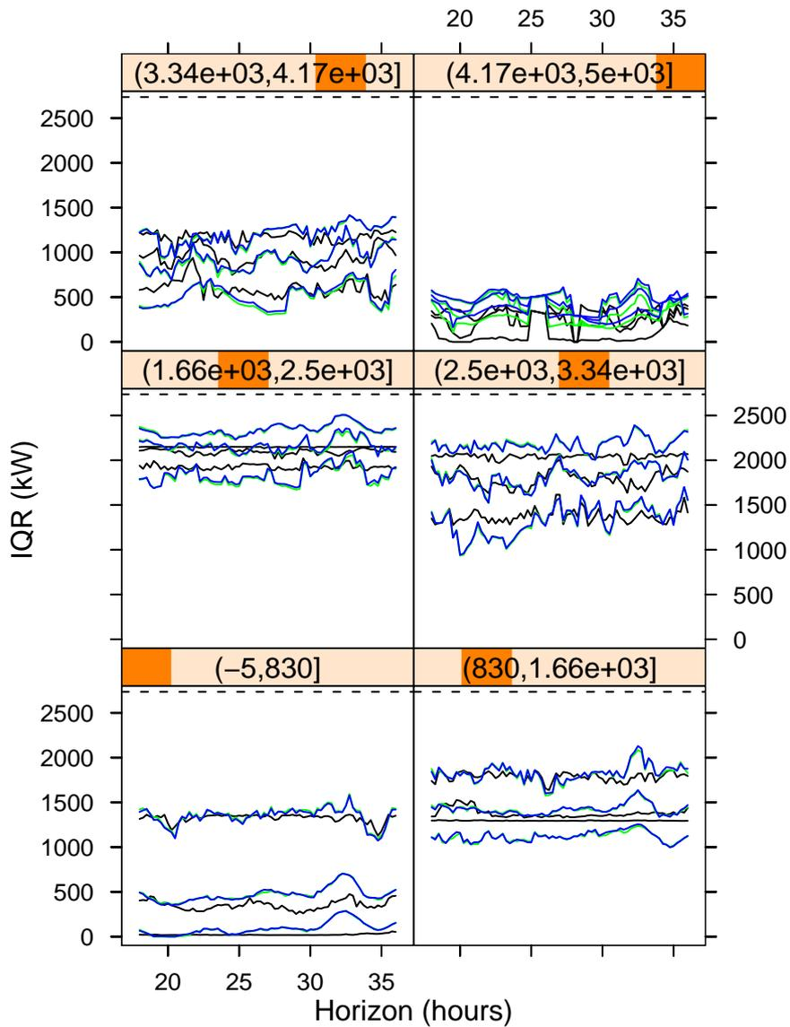
**Figure 4.9:** Quantiles (5%, 50%, 95%) of the inter quartile range (IQR). Models: Basic (black), w/o density (green), incl. risk (blue). The grouping variable is the power production (kW) as forecasted by WPPT and split in six intervals of equal length. The horizontal line at 2736 kW indicate the IQR of actual power productions between 1/7-1999 and 1/6-2003.
