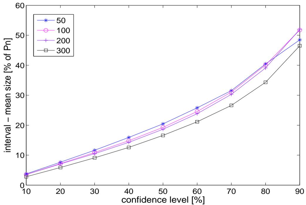
Figure 5.12:  $\delta$ -diagrams for 24-hour ahead forecasts for evaluating the influence of the error sample size on the resulting probabilistic forecasts' sharpness.
