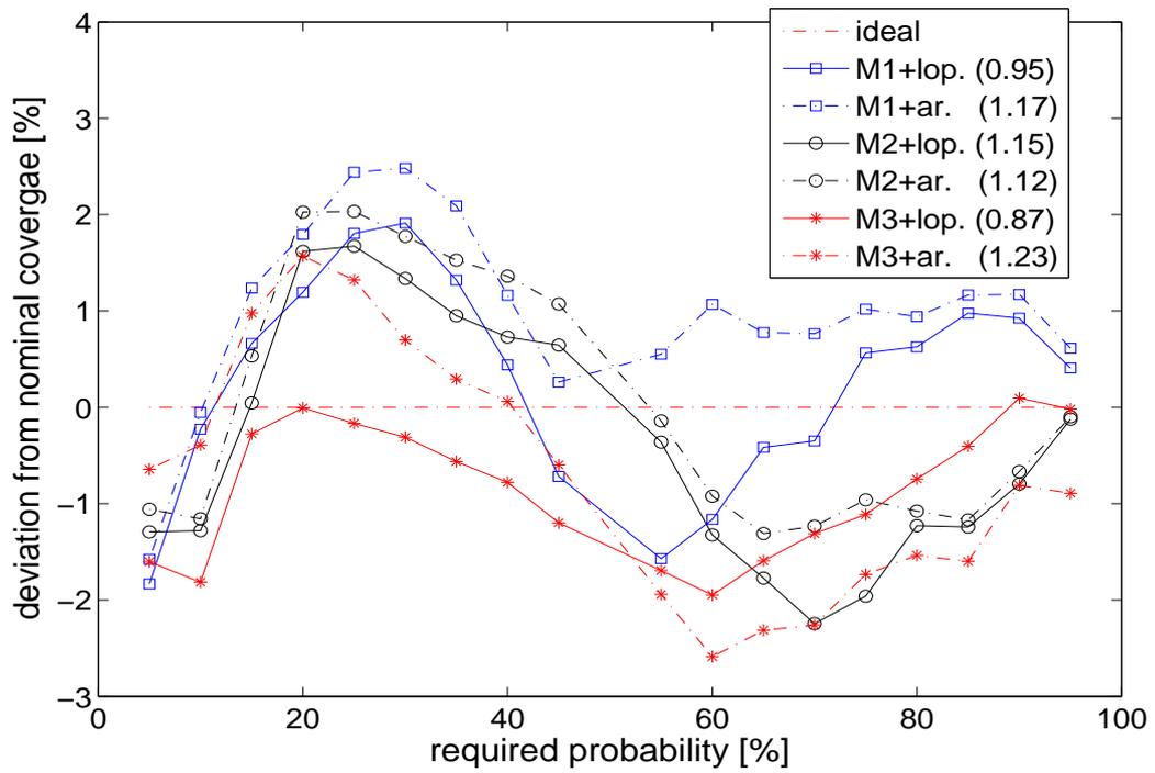
Figure 5.5: Reliability diagrams for Tunø Knob. Results are given for the three point prediction methods and for the two implemented approaches (lop: linear opinion pool; ar: adapted resampling).
