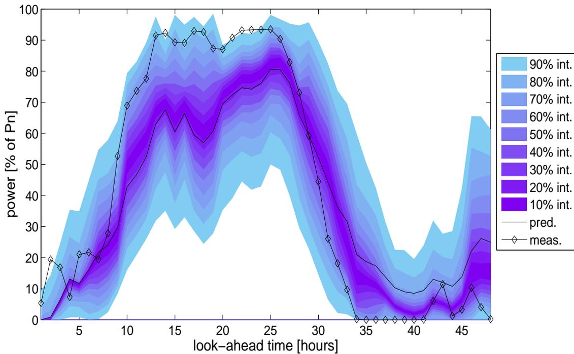
**Figure 5.4:** Example of wind power point predictions associated with a set of interval forecasts. The point predictions are given by M2 and the central interval forecasts are estimated consequently with the adapted resampling method. Nominal coverage rates range from 10 to 90%. These sets of predictions and intervals were issued on the 28<sup>th</sup> March 2003 at 10:00, for the Tunø Knob wind farm.
