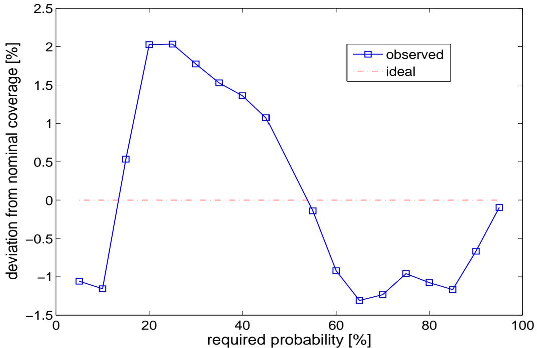
**Figure 5.3:** Example of a reliability diagram depicting deviations as a function of the nominal coverage rate, for the reliability evaluation of a method providing probabilistic forecasts of wind generation.
