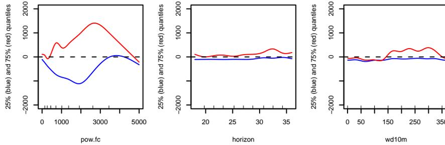
**Figure 4.5:** Estimated 25% (blue) and 75% (red) quantiles when excluding the forecasted air density from the model. The rugs on the 1st axis in the top row of plots indicate the placement of knots.
