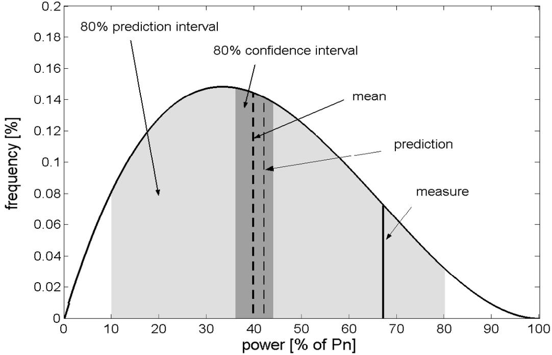
**Figure 5.1:** Illustrative example of the difference between confidence (light shaded area) and prediction (dark shaded area) intervals. The confidence interval is a measure of the confidence in our estimate  $\hat{p}_{t+1/t}$  of the expectation  $\bar{p}_{t+1}$ , whereas the prediction interval is related to the accuracy of the point forecast  $\hat{p}_{t+1/t}$  with respect to the true effect  $p_{t+1}$ .
