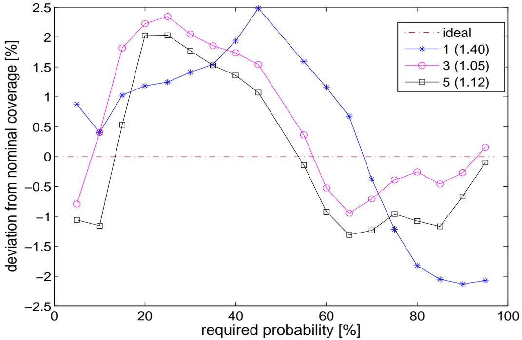
Figure 5.9: Reliability diagrams for evaluating the influence of the power curve mapping on the resulting probabilistic forecasts' reliability.
