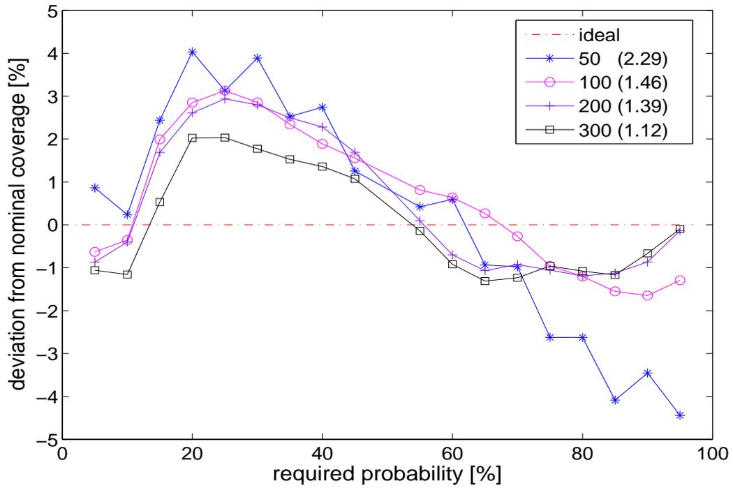
Figure 5.11: Reliability diagrams for evaluating the influence of error sample size on the resulting probabilistic forecasts' reliability.
