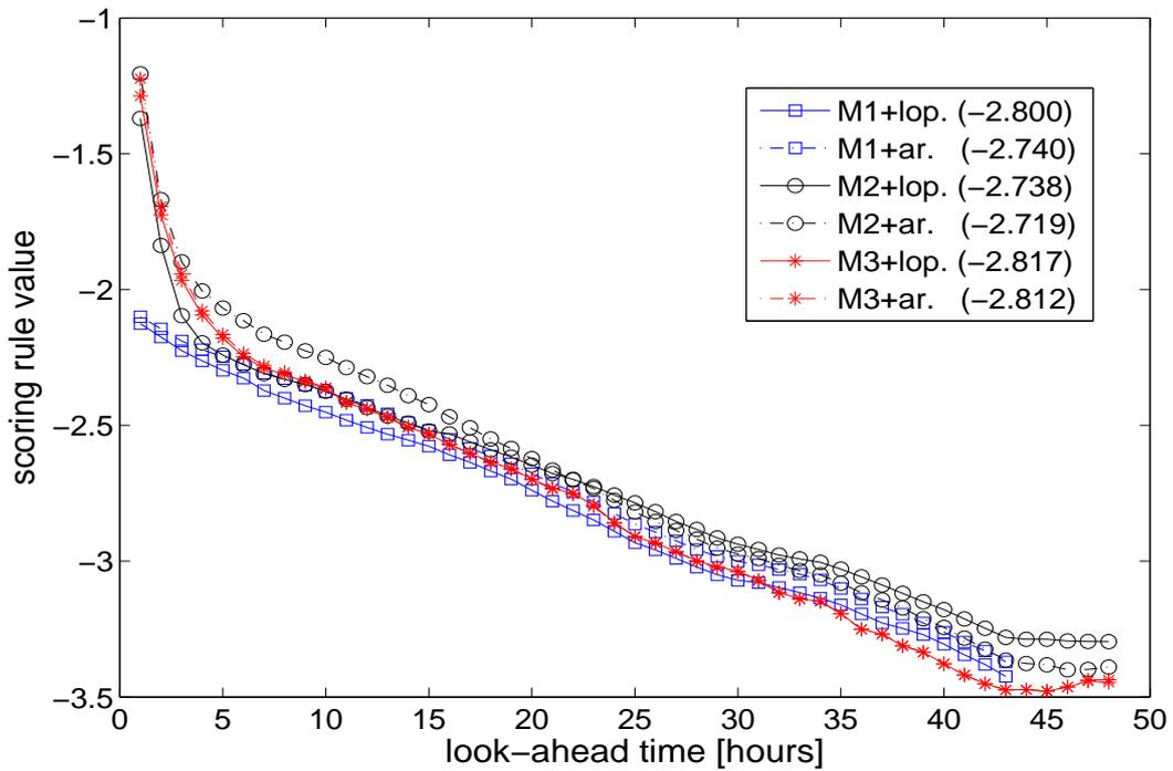
Figure 5.8: Skill score as a function of the horizon for Klim. Results are given for the three point prediction methods and for the two implemented approaches (lop: linear opinion pool; ar: adapted resampling).
