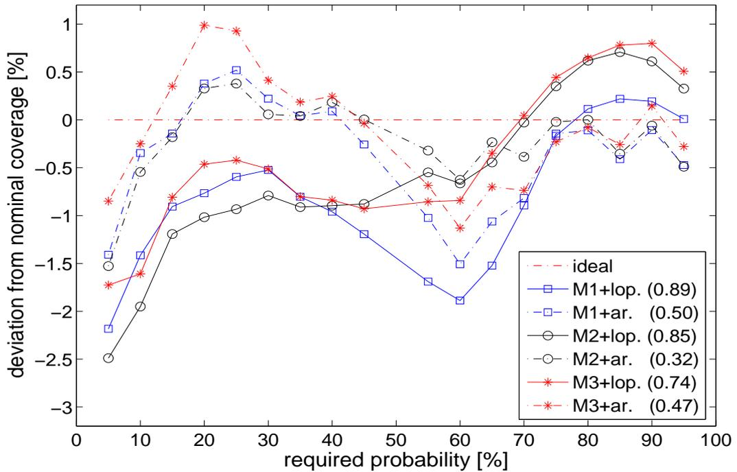
Figure 5.6: Reliability diagrams for Klim. Results are given for the three point prediction methods and for the two implemented approaches (lop: linear opinion pool; ar: adapted resampling).
