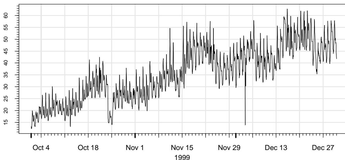
Figure 5.1: Hourly heat demand in  $MW$  for the last quarter of 1999.
