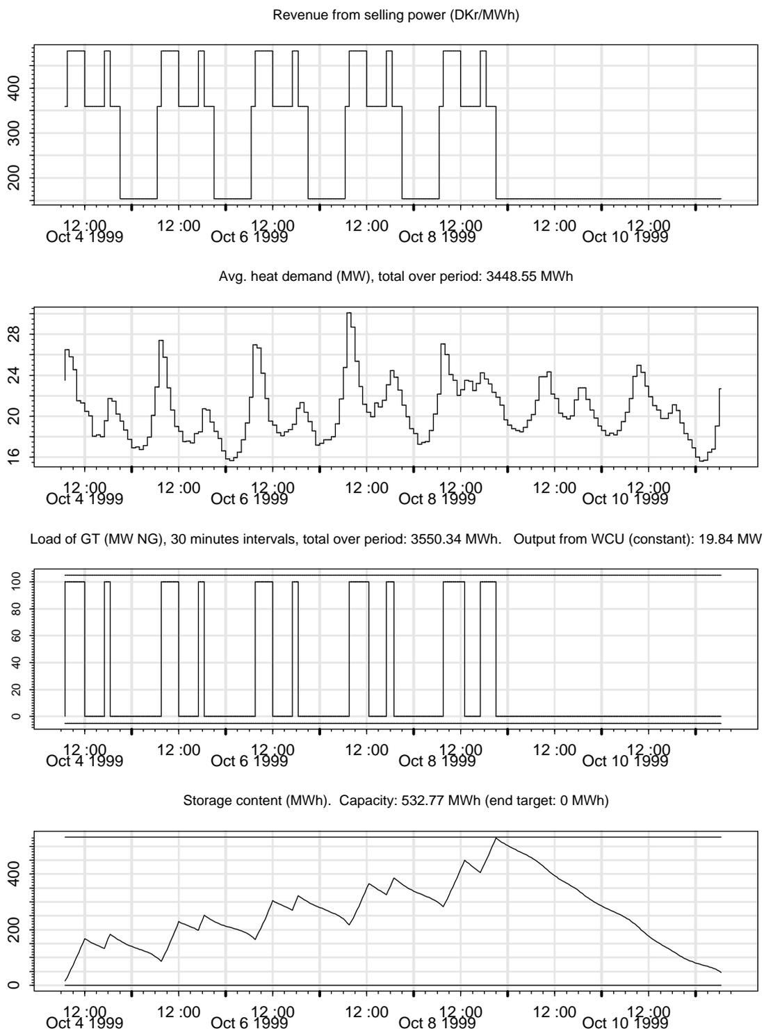
Figure 5.2: Optimal operation of gas turbine for one week starting on 1999.10.04 (criteria function: 612526 *DKr*).
