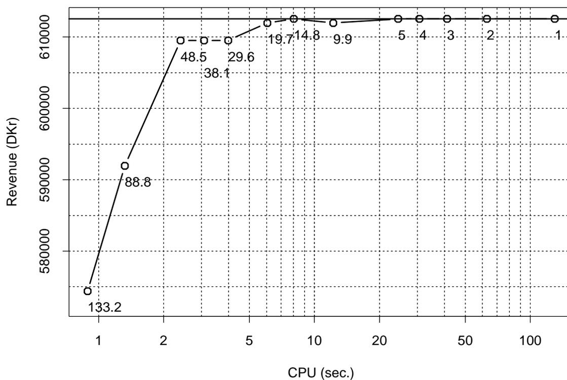
Figure 5.6: Revenue versus seconds of CPU time used on a PC with a 450  $MHz$  Pentium III processor running Linux for varying degrees of discretization as indicated below each point ( $MWh$ ). The horizontal line indicates the revenue obtained using steps of 0.1  $MWh$  (approx. 24 min.). The optimization problem is the one considered in Figure 5.2. Note the log-scale on the horizontal axis.
