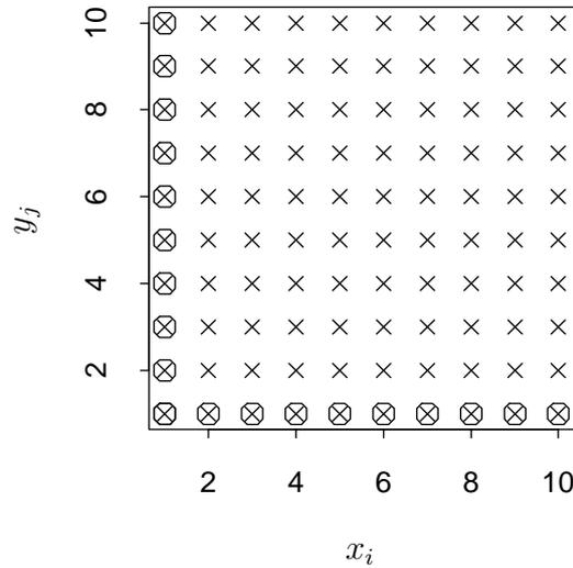
Figure 3.2: Points needed for an additive model ( $\circ$ ) and a non-additive model ( $\times$ ).
