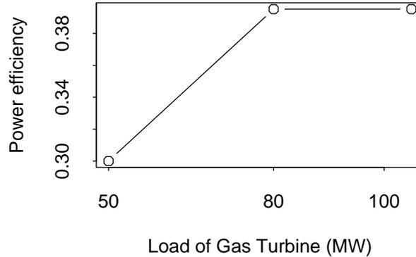
Figure 6.1: Assumed efficiency of producing power ( $\eta_{gp}$ ) on the gas turbine against the load of the gas turbine ( $F_g$ ).
